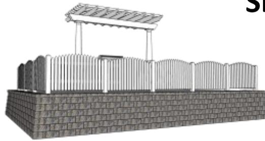
The core should be filled to 3/4 of an inch from the top of the wallstone. Place the correct select backfill soil as advised by engineer and compact. Use only lightweight compaction equipment within 3 feet of the back of the Sigma 8-Inch Wall. Sweep the top of the wallstones clean before adding the next layer.
